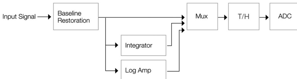
Figure 1 – Analog Track and Hold Block Diagram
