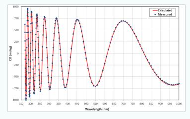
**DichOS** produces a CD spectrum comprising multiple peaks from the Far-UV to the NIR (see left). The model spectrum (red) can be calculated very precisely and this is compared with the measured spectrum (blue).
