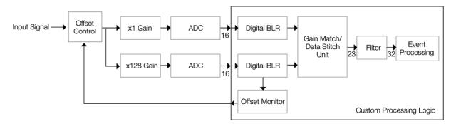
Figure 5 - Multi-Gain Adaptive Block Diagram
