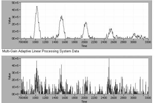
The combination of gain stages and stitching techniques provides a very high dynamic range with very high resolution. For comparison, a system with only one ADC was tested along with a Multi-Gain Adaptive Linear Processing system. Each system was connected to exactly the same input source, with the input being a series of 5 pulses linearly distributed from 1mV to 100uV. Data from this test is shown in Figure 6, with graphs having the same scale.
