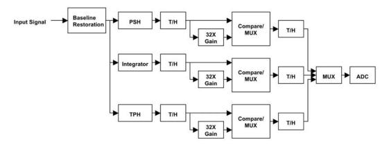
Figure 2 – Analog/Digital Hybrid Block Diagram
