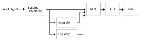
Figure 1 – Analog Track and Hold Block Diagram
